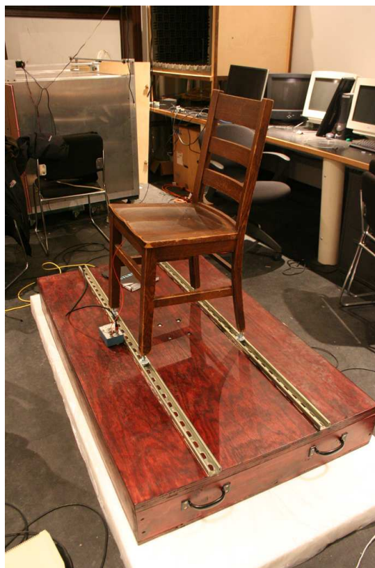
Fig. 3: Motion platform used in multimodal presentation of audio-tactile stimuli. Sennheiser HD280 headphones are used for audio presentation.
