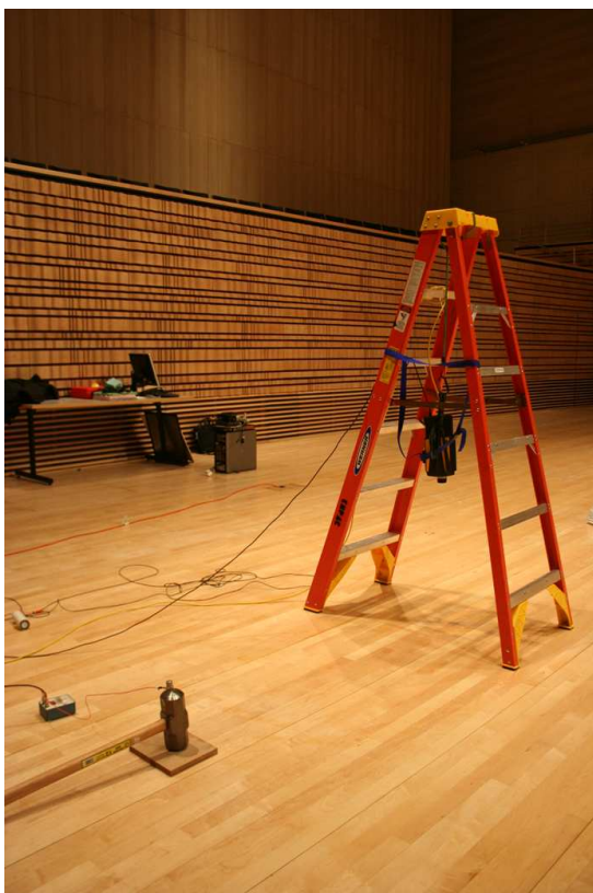
Fig. 2: Structural impulse response measurement equipment. Instrumented sledgehammer used to measure force input, laser doppler vibrometer used to measure force output (isolated from the stage with a bungee cord). Not Shown: 68-kg sand bag placed on a chair used to mass load receiver position. The source position is mass loaded by an experimenter operating the sledgehammer.
